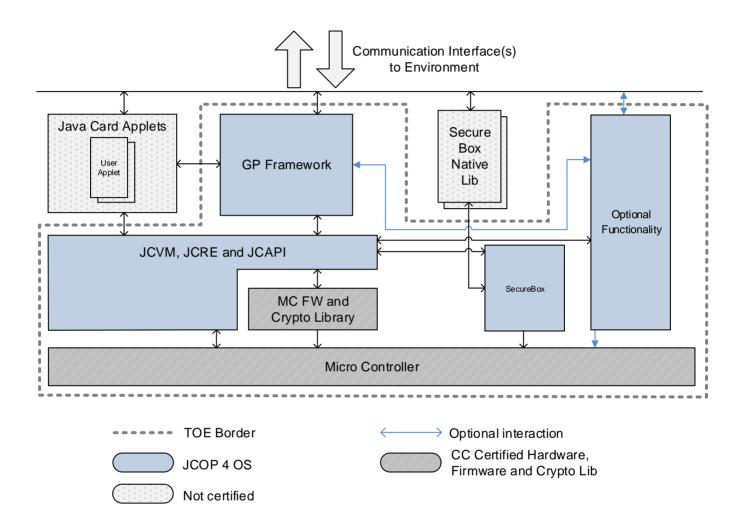
Fig. 1.1: Components of the TOE
